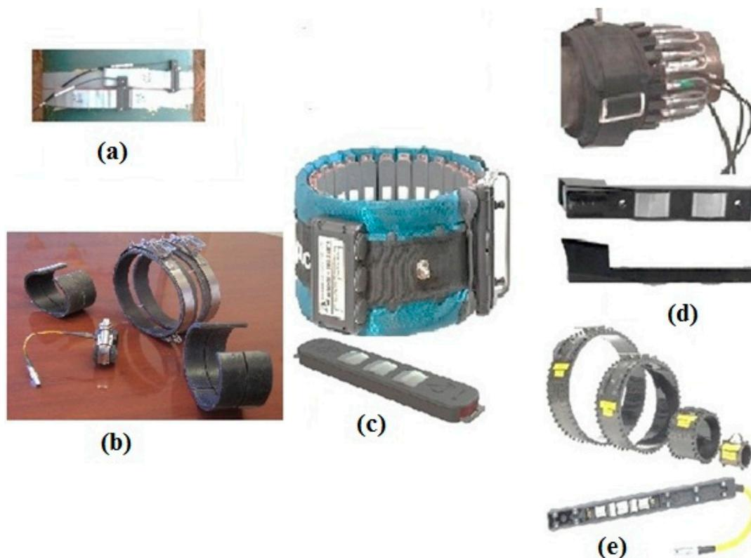
**Figure 9.** Commercially available collar and its transducers: (a) a US-based MsSR3030 transducer (Guided Wave Analysis LLC, San Antonio, TX, USA) [175]; (b) a set of magnetostrictive transducers made for high temperatures [166]; (c) a UK-based collar and its transducers (Guided Ultrasonics Ltd., London, UK) [176]; (d) a Japan-based collar and its transducers (Olympus Co., Tokyo, Japan) [177] and (e) a UK-based collar and its transducers (Teletest<sup>®</sup> Focus, Cambridge UK) [178].
