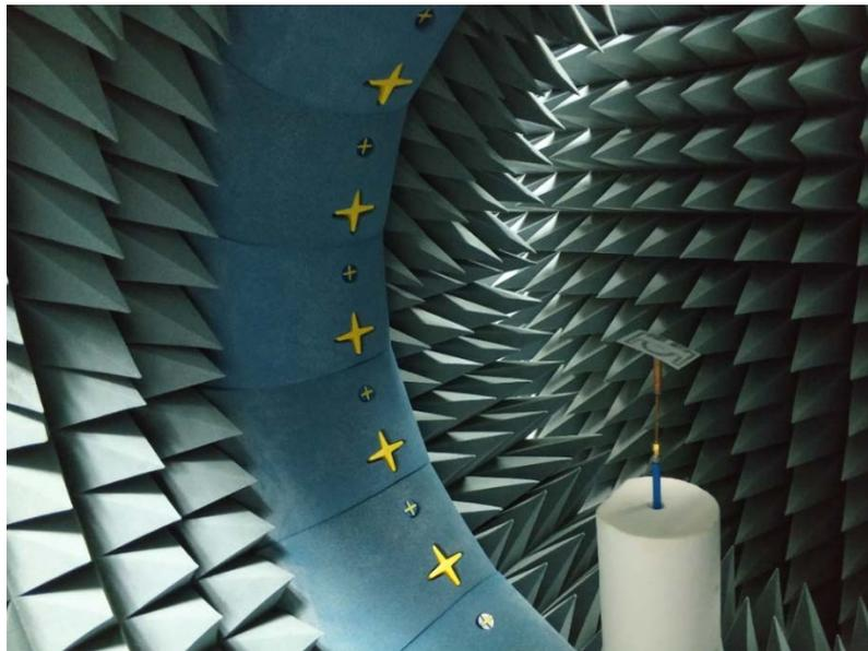
Figure 4. Far-field characteristics measurement using a Satimo near-field measurement system.
