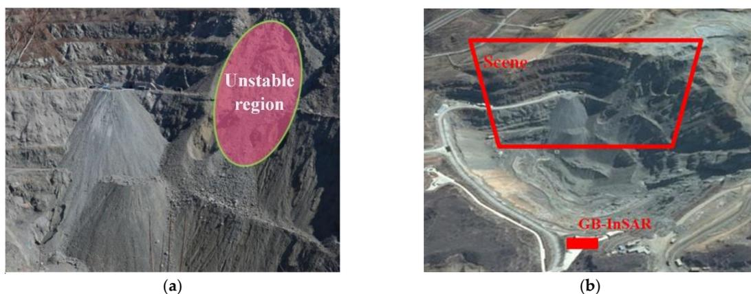
**Figure 5.** Deformation monitoring for case study 1: (a) the optical photo and (b) the aerial view on Google Earth.
