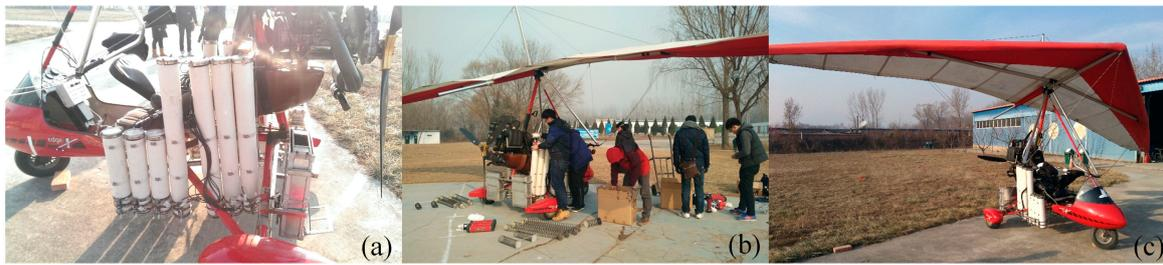
**Figure 12.** Preparation for the integrated demonstration: (a) Equip airplane with launch cabins. (b) Load ground robots, separation devices, and parachutes into launch cabins. (c) Preparation is done.
