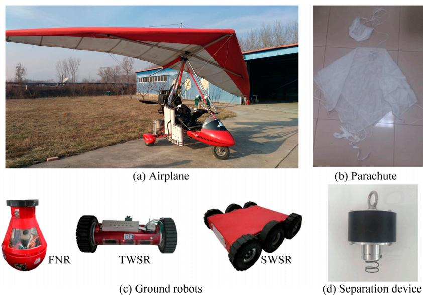
**Figure 9.** Experimental platform of MSADM.
