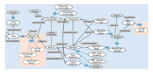
Figure 6. Modified oneM2M Base Ontology for VO design.
