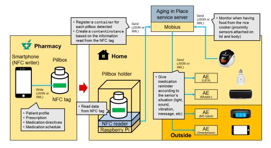
**Figure 15.** The overall diagram for the service scenario for medication reminder service using aging in place (AIP) service platform, smart pillbox kit, and various IoT products.
