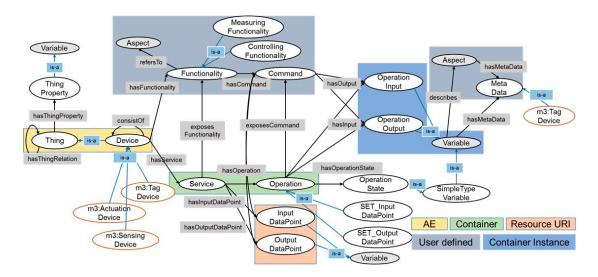
Figure 5. oneM2M resource mapping with oneM2M Base Ontology for Virtual Object (VO) creation.
