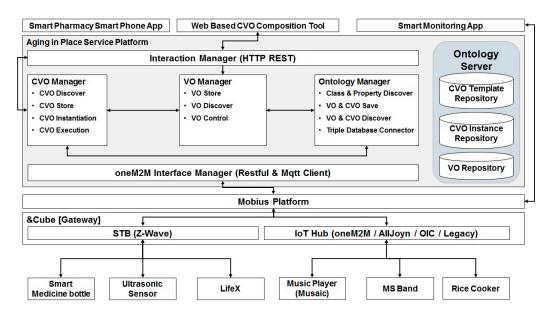
Figure 4. System architecture of aging in place (AIP) service platform.
