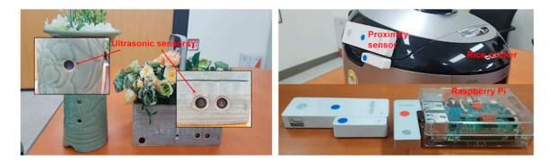
Figure 18. Ultrasonic sensors (left) and rice cooker embedded with proximity sensors (right).
