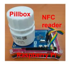
**Figure 16.** The pillbox with an NFC tag (**left**) and pillbox holder (**right**) consisting of a Raspberry Pi and NFC reader.
