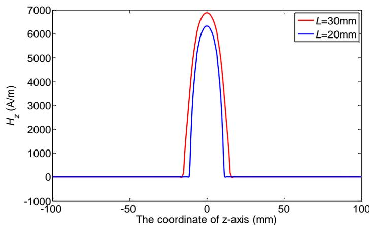
Because of the existence of the two copper rings, the axial lengths of the alternating magnetic fields are both close to  $L$  under two different conditions. Besides, the shapes of distributions are much more similar than the conventional structure as shown in Figure 5. Therefore, the special structure can be used to study the relationship between the axial length of alternating magnetic field and the excitation efficiency.
