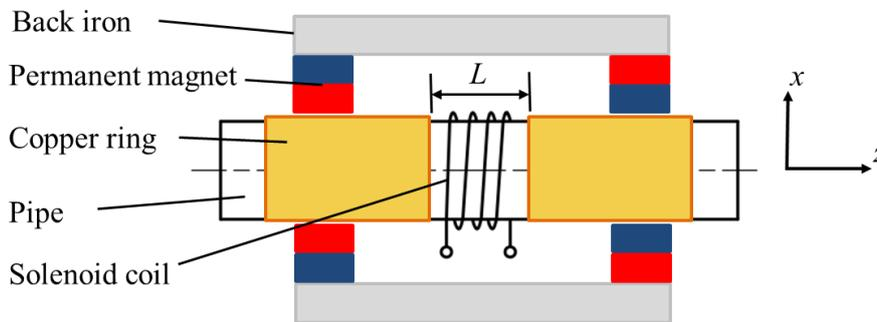
Figure 8. The alternating magnetic field produced by the special structure when  $L = 30$  mm.
