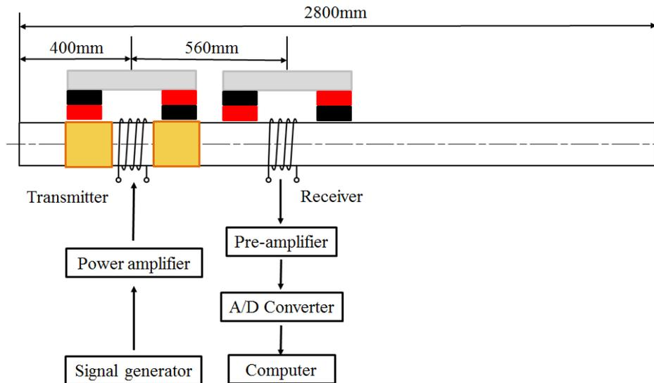
The amplified sine pulse current is provided to the transmitter coil. The received voltage signal of the receiver coil is amplified by a pre-amplifier, then digitized and sampled by a 16-bits data acquisition card and finally interfaced to a computer.
