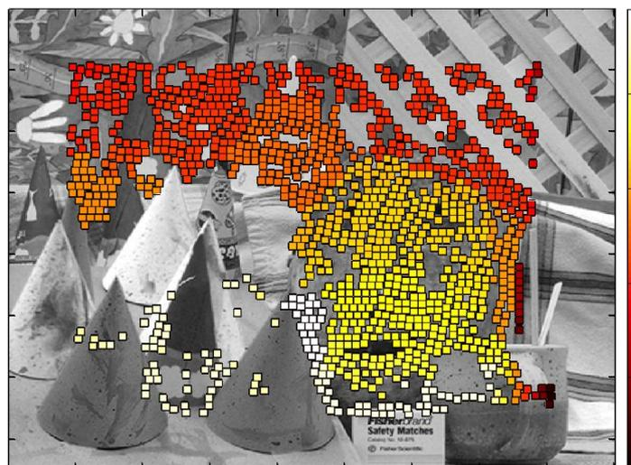
The stereo flow is injected directly from an external memory connected to the FPGA. This real emulation allows considering any stereo system regardless of the source image used, without taken care about other aspects such as control of camera lines and parameters of image capture. This dense map could give up to 30,000 data points using the configuration presented above.
