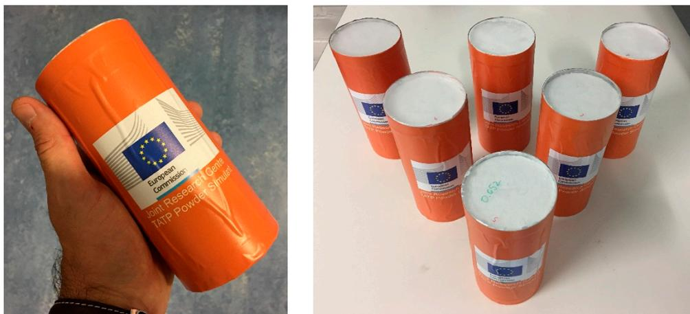
**Figure 2.** Photos of our TATP simulant based on stearates, caffeine and benzoates.
