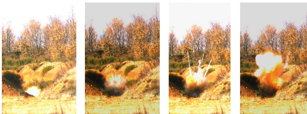
**Figure 7.** Detonation sequence of bulk TATP recorded with a high-speed camera at the INTA test site near Leon, Spain.
