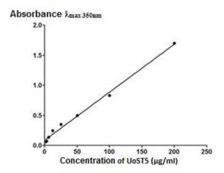
Supplementary Figure 1. Calibration curve for the dilution series of UoST5 at  $\lambda_{max\,350}$  showing linearity over concentration range of 3.125-200 µg/ml .The maximum absorbance ( $\lambda_{max}$ ) was determined by UV/VIS spectrophotometer then serial dilution of UoST5 in DCM was prepared and measured at  $\lambda_{max}$  using DCM as sample blank.
